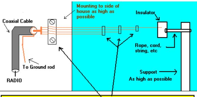
This insulator/strain relief is used to keep strain off the connection. It can be made from a simple strip of wood pressed over the 4 wires using one twist around it and then screwed to the house. You can experiment with your particular mounting. Since the longest wire will be the main support for the other 3 shorter wires, you will have to secure each shorter wire to the longer wire to support them. Use electrical tape or your own method making sure none of the wires short to any other wire.
