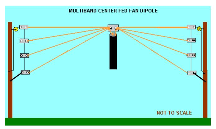
Shown supported between two wooden poles. Gray rectangles are insulators. Yellow circles are pulleys.
